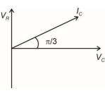
Current lead voltage by  $\frac{\pi}{3}$  therefore alternating
